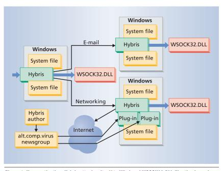
Figure 1. Upon activation, Hybris attaches itself to Windows' WSOCK32.DLL file, the dynamic link library that implements an application's Windows Socket API. Hybris uses Windows Sockets functions to scan e-mail addresses that victims receive and Web pages they visit. Hybris then spreads by e-mailing itself to the victims' addresses. Hybris can also connect via the Internet to the alt.comp.virus newsgroup to update its malicious capabilities.
